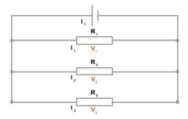
a i R<sub>1</sub> has a resistance of 5 ohms. The current flowing in it is 2A. Calculate the potential difference across R<sub>1</sub>.
