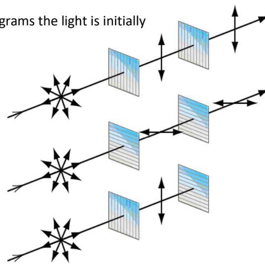
\* In the bottom diagram the light becomes vertically polarized but this cannot pass through a horizontal plane Polaroid.
