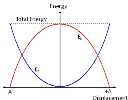
For a mass on a spring there is a transformation between kinetic energy, gravitational potential energy and the energy stored in the spring (elastic potential). At the top there is maximum elastic and gravitational but minimum kinetic. In the middle there is maximum kinetic, minimum elastic but it still has some gravitational. At its lowest point it has no kinetic, minimum gravitational but maximum elastic.
