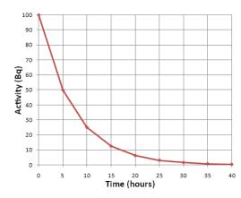
We can calculate the half-life from activity and number of nuclei graphs. Choose a starting value and then find how long it takes to fall to half this value. In the graphs we can see that both fall from 50 to 25 and take 5 hours to do this. Therefore the half-life is 5 hours. Knowing this we can then calculate the decay constant.
