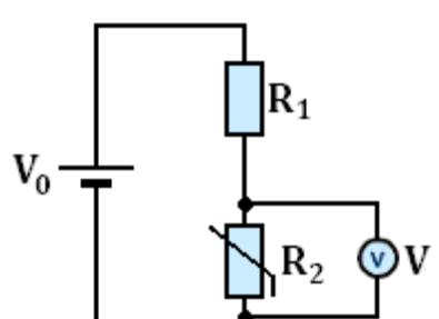
output voltage low. A use of this would be a cooling fan that works harder when it is warm.
