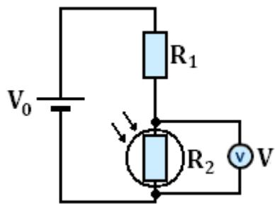
In the second potential divider the second resistor is a Light Dependant Resistor. When the light levels are low the resistance ( $R_2$ ) is high, making the output voltage high. When the light levels increase the resistance ( $R_2$ ) decreases, this makes the output voltage decrease. A use of this could be a street light sensor that lights up when the surrounding are dark.
