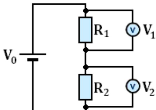
A potential divider is used to produce a desired potential difference, it can be thought of as a potential selector.
