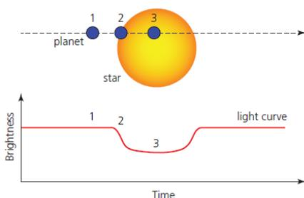
The Transit Method: This works by detecting a dimming in the star's brightness as an exoplanet moves across its disc, perpendicular to our line of sight – called a transit. The decrease in observed brightness allows the radius of the exoplanet to
