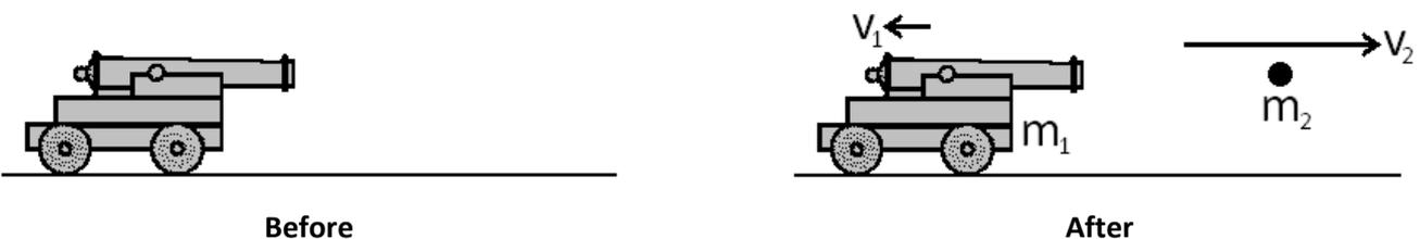
If we look at the example above we can see that the whole system is not moving, so the momentum before is zero. After the explosion the shell travels right with velocity  $v_2$  and the cannon recoils with a velocity  $v_1$ .
