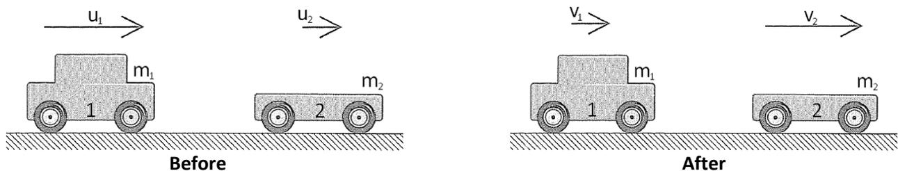
In the situation above, car 1 and car 2 travel to the right with initial velocities  $u_1$  and  $u_2$  respectively. Car 1 catches up to car 2 and they collide. After the collision the cars continue to move to the right but car 1 now travels at velocity  $v_1$  and car 2 travels a velocity  $v_2$ . [ $\rightarrow$  is positive]
