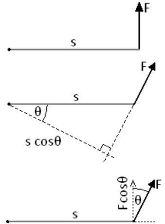
**Moments are measured in Newton metres, Nm**
