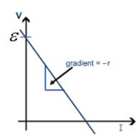
Graphs have the general equation of y = mx+c, where y is the vertical (upwards) axis, x is the horizontal (across) axis, m is the gradient of the line and c is where the line intercepts (cuts) the y axis.
